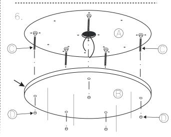
Remove rods and attach  $\bigcirc$  to  $\bigcirc$  with the button head screws  $\bigcirc$
